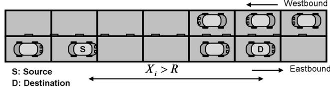
(a) At  $t=0$ , adjacent cells are unoccupied and the network is disconnected.
