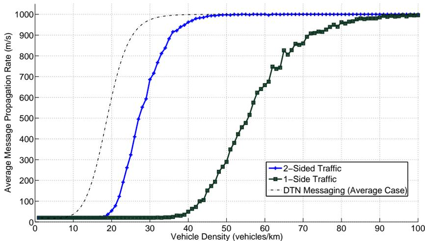
Figure 13: Simulation results – Comparison of DTN Messaging Strategy with a path formation based scheme utilizing 1-sided traffic and both sides of traffic for a distance of 12.5Kms.
