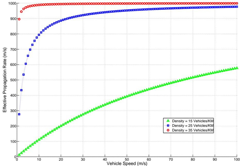
Figure 14: Simulation results – Comparison of impact of increasing density on effective propagation rate for various values of vehicular speed.
