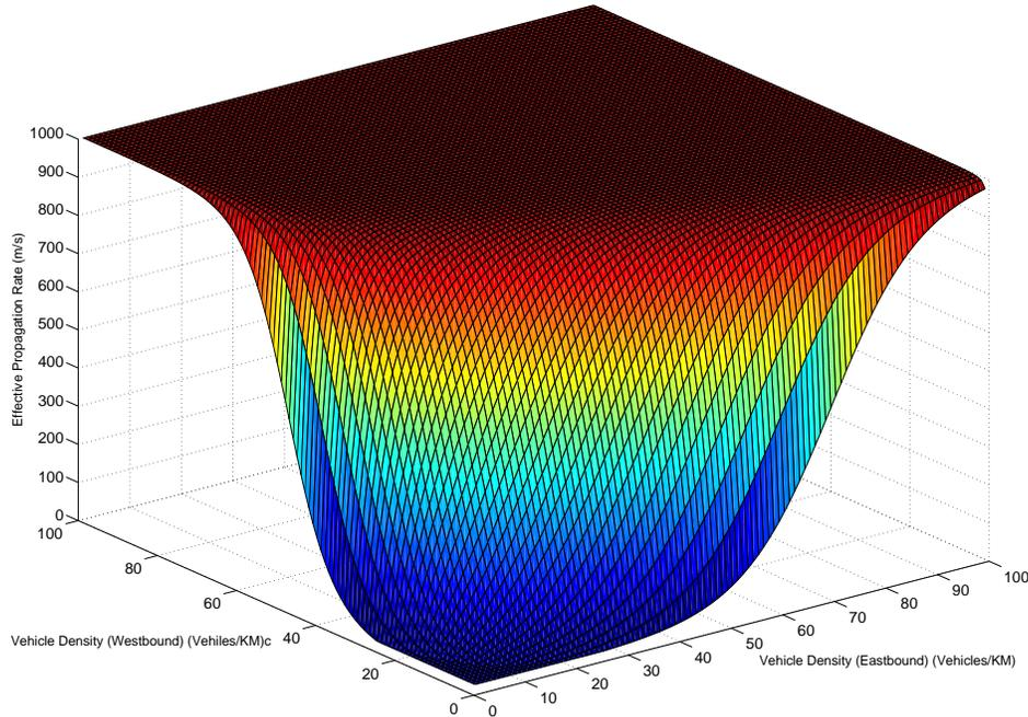
Figure 11: Simulation results – Results for Message Propagation Rate as a function of various *Eastbound* and *Westbound* vehicular traffic densities.
