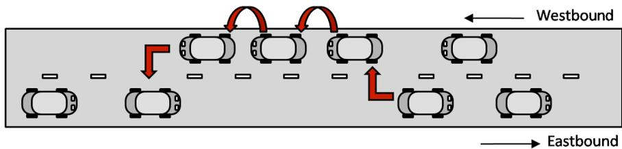
Figure 4: Partitions are bridged using vehicles traveling in the opposing direction.
