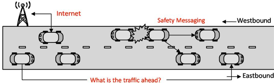
Figure 2: Three classifications of data exchange in vehicular networks.
