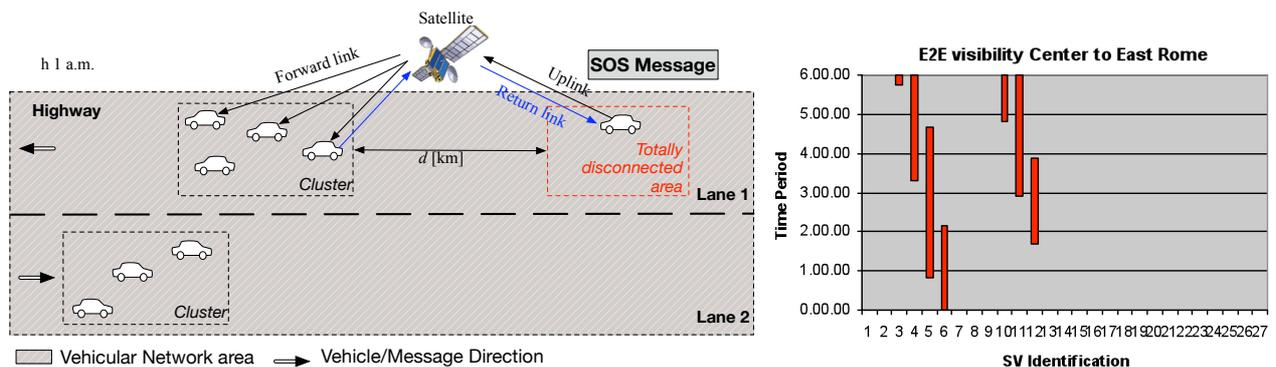
Figure 1. (*left*) Novel opportunistic networking scheme in a VANET scenario with satellite connectivity for safety applications. (*right*) Forward link end-to-end (E2E) visibility, Rome city vs. East Rome.
