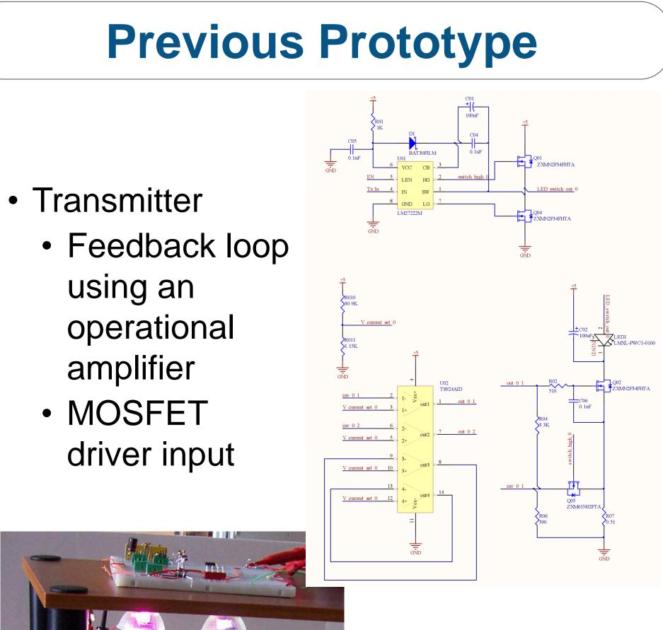
both the transmitter and receiver on the same board, allowing for two-way communications.
