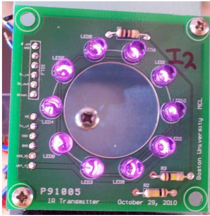
The VLC-infrared (VLC-IR) transceiver: •eliminates optical crosstalk between uplink and downlink
