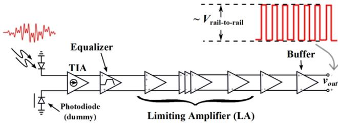
Figure 6: Conventional optical receiver based on limiting amplifier (LA) (Offset cancellation network not shown).
