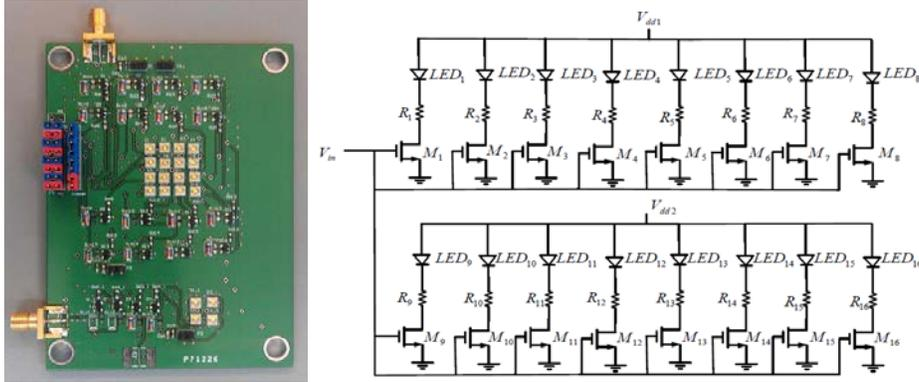
Figure 10: Analog LED driver (left) and circuit (right).
