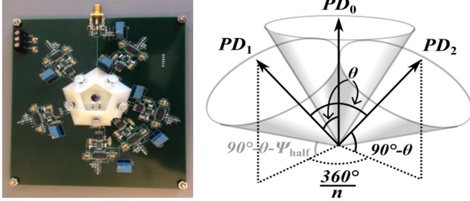
Figure 12: Diversity receiver (left) and the FOV design model for an arbitrary  $n$  (right).
