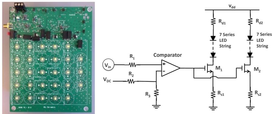
Figure 11: Two-level LED driver (left) and circuit (right).
